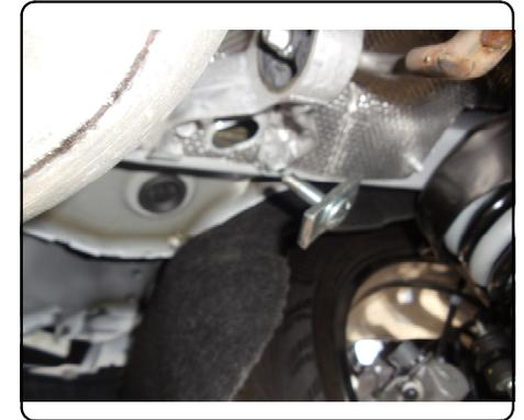
2. Place hitch underneath vehicle and route fishwire through side plate mounting holes. It may be necessary to use two people to raise the hitch into position. Remove fishwire and loosely secure mounting hardware to hold the hitch into position.
