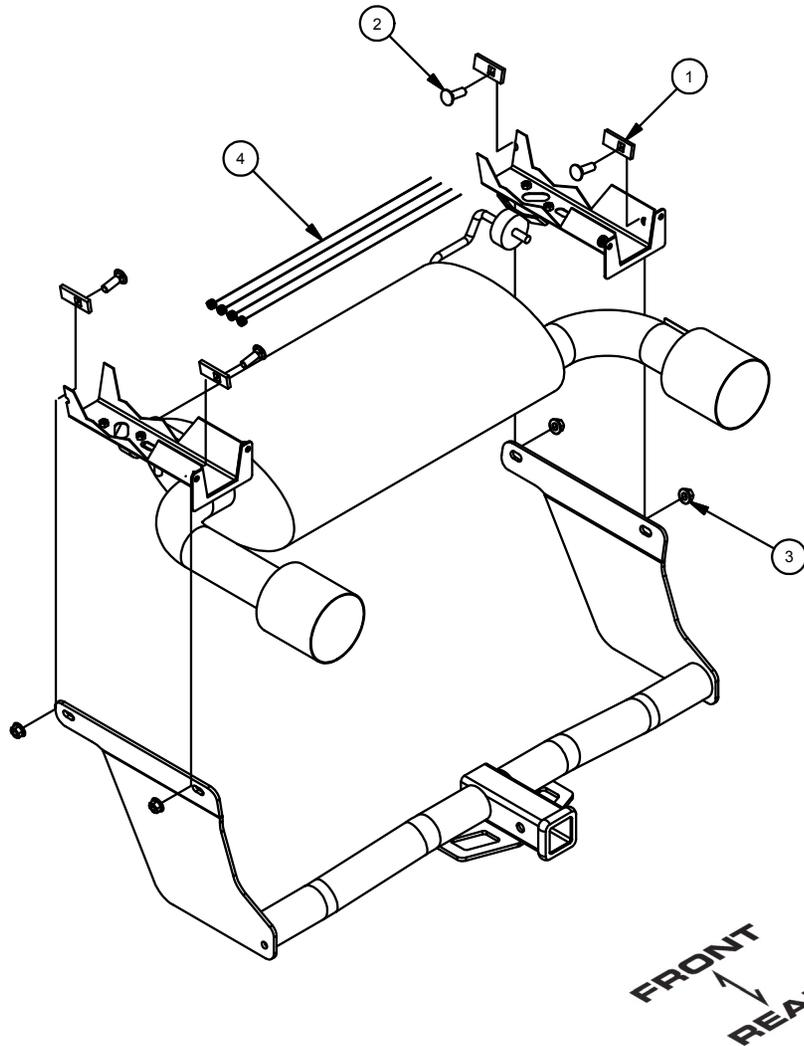
1. Enlarge access holes for square hole spacers with a die grinder.
